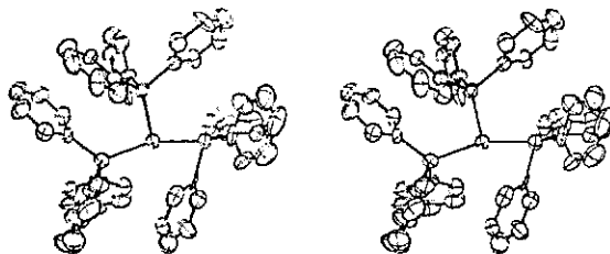
Fig. 15.48 Stereoview of the structure of the [(\text{Ph}_3\text{P})_3\text{Rh}]^+ cation, showing the planar, approximately T-shaped coordination about the rhodium atom. Note the unusual manner in which the phenyl ring at the lower right is drawn toward the rhodium atom. [From Yared, Y. W.; Mites, S. L.; Bau, R.; Reed, C. A. J. Am. Chem. Soc. 1977, 99, 7076-7078. Reproduced with permission.]
