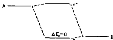
Fig. 5.23 Heteronuclear molecule, A^+B^- , with large electronegativity difference. Covalency is insignificant; the bond is essentially ionic.
